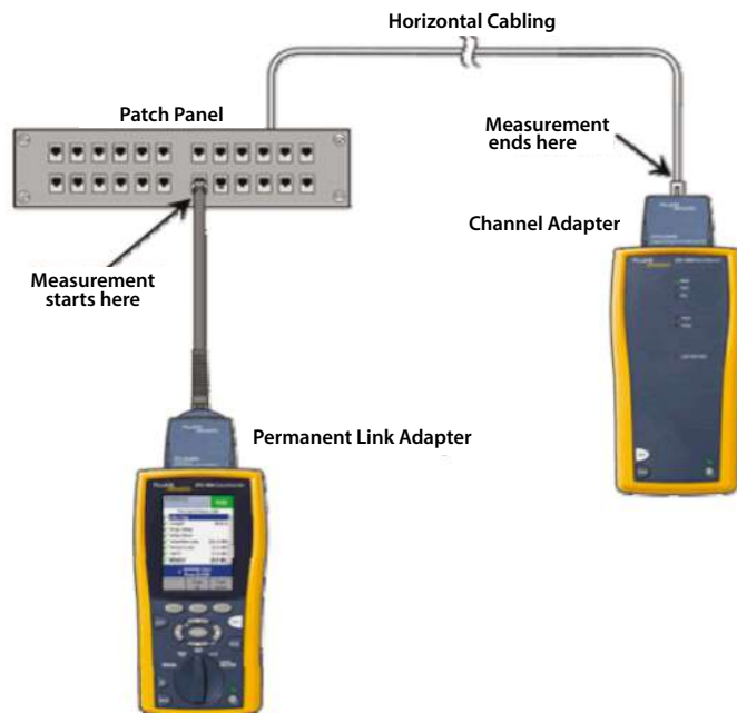
* Remote channel adapter & RJ45 plug are excluded from the measurement using Digital Signal Processing
